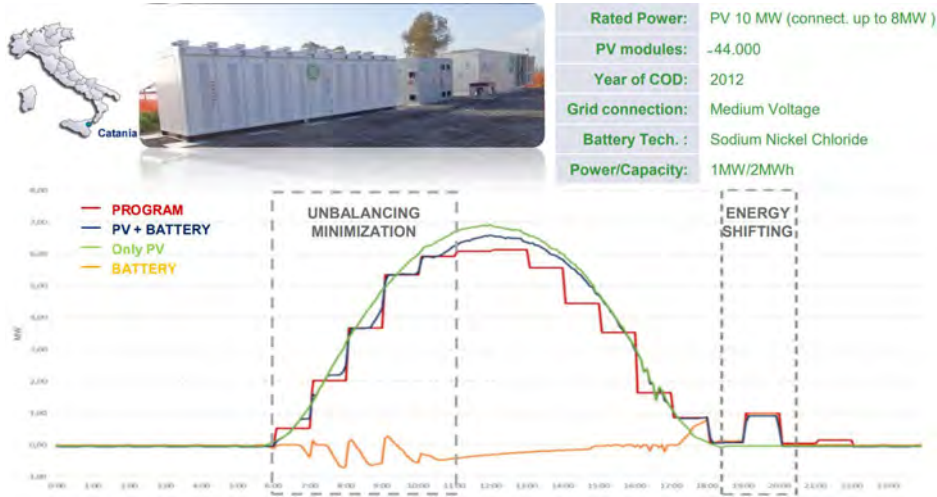
Figure 3.5: Solar Photovoltaic Installation with a Storage System
