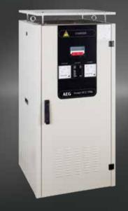
The Protect RCS TPRE TD battery charger system has been developed and designed to provide high reliability power supply and battery charging capability. The Protect RCS TPRE TD is a thyristor-controlled battery charger suitable for charging nickel-cadmium or lead-acid batteries while supplying DC loads. Its design is optimized for T&D (Transmission and Distribution) applications.
