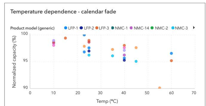
Figure 5-5 Temperature dependence of calendar fade degradation across various cells
