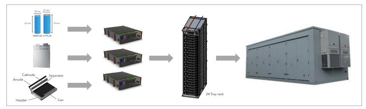
Figure 4-1 UL9540A testing is conducted at the cell, module, unit (racks), and installation (system) level
