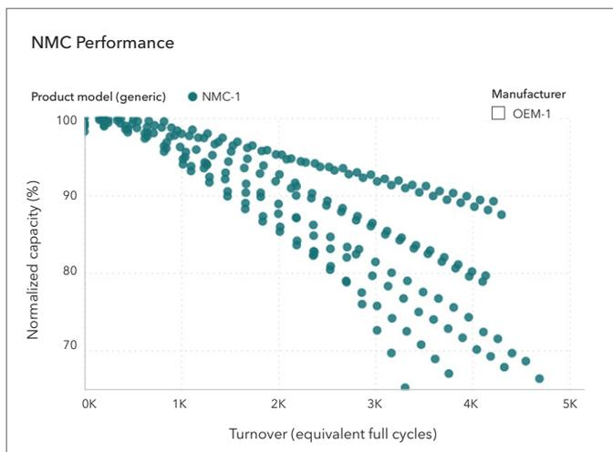
Figure 5-3 Top performing cells in the EV/high C-rate category
