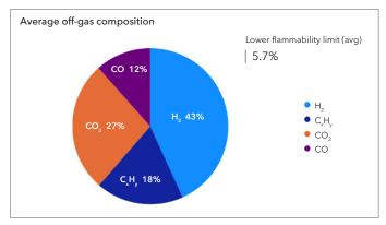
Figure 5-8 Off-gas composition of gas released during thermal runaway
