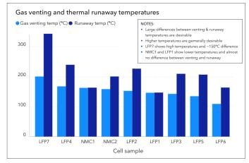
Figure 5-7 Venting and thermal runaway onset temperatures for various cells across chemistries
