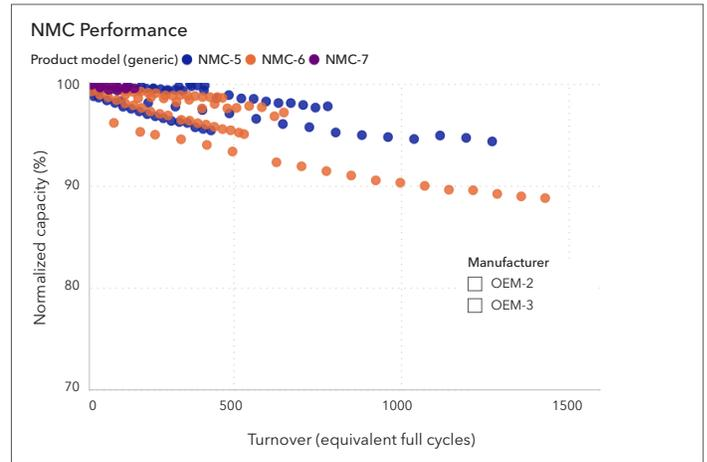
Figure 5-2 Top 3 performing cells in the 4-hour solar shifting category
