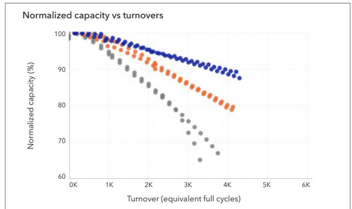
Figure 5-6 Degradation rates can be significantly affected by adjusting the upper voltage limit in the BMS
