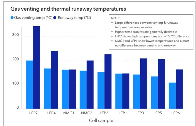
Figure 5-7 Venting and thermal runaway onset temperatures for various cells across chemistries
