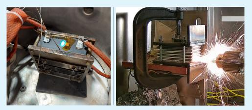
Figure 4-2 Cell-level testing helps understand failure modes and thresholds of each battery cell
