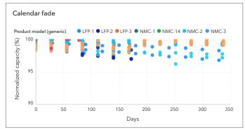
Figure 5-4 Calendar fade degradation at room temperature across various cells and at 30% and 100% SOC
