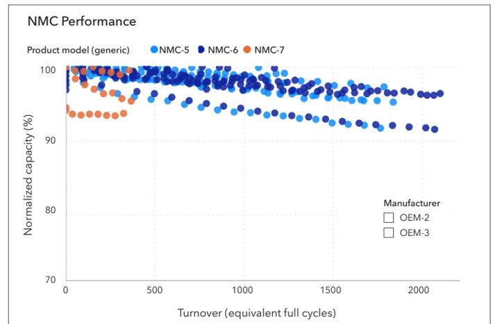
Figure 5-1 Top 3 performing cells in the <2 hour grid support category
