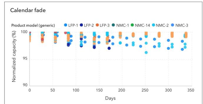
Figure 5-4 Calendar fade degradation at room temperature across various cells and at 30% and 100% SOC
