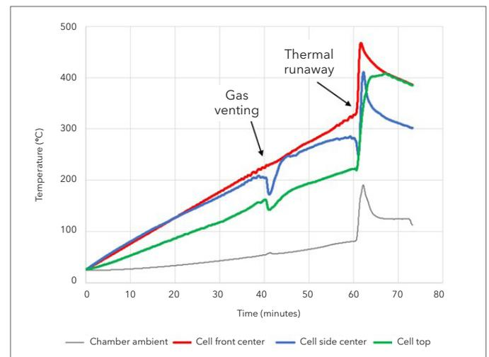
Figure 4-3 Cell-level UL 9540A test results show temperatures rising steadily, dipping, rising again, and then spiking during thermal runaway
