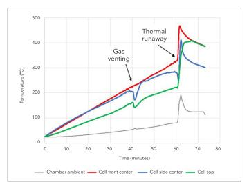
Figure 4-3 Cell-level UL 9540A test results show temperatures rising steadily, dipping, rising again, and then spiking during thermal runaway
