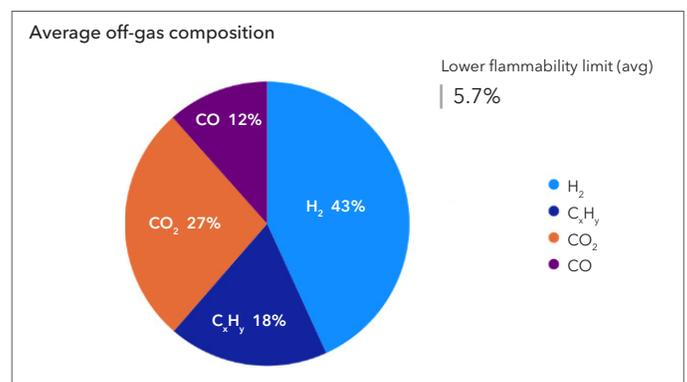
Figure 5-8 Off-gas composition of gas released during thermal runaway
