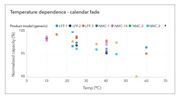
Figure 5-5 Temperature dependence of calendar fade degradation across various cells
